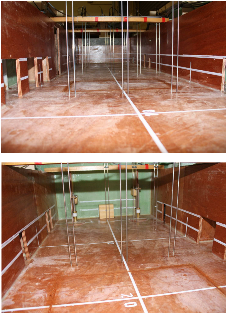
Figure 15: Wave probes inside the hold
