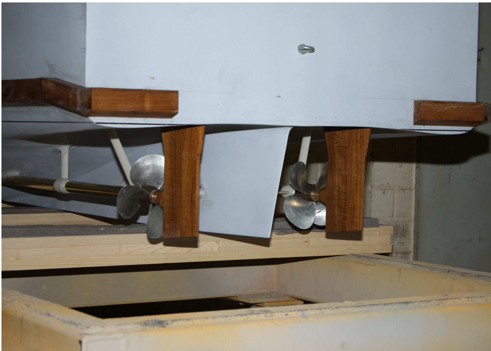
Figure 12: Rudder and propeller arrangement
